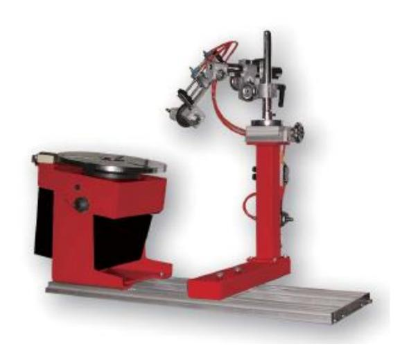
BASIC SYSTEM COMPRSING OF POSITIONER UNIT AND TORCH HOLDER. AVAILABLE IN A VARIETY OF BED LENGTHS TO SUIT THE COMPONENT.
