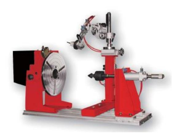
TAILSTOCK SYSTEM COMPRSING OF POSITIONER UNIT AND TORCH HOLDER. AVAILABLE IN A VARIETY OF BED LENGTHS TO SUIT THE COMPONENT. VARIOUS CHUCK SIZES FOR DIFFERNET DIAMETERS ALSO AVAILABLE
