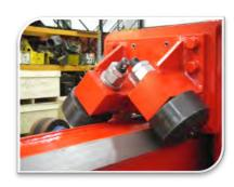
HEAVY DUTY BEARINGS. MACHINED SLIDEWAYS FOR SMOOTH BOOM ARM TRAVERSE AND CARRIAGE ELEVATION
