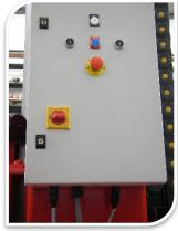
COLUMN MOUNTED CONTROL BOX WITH IDENTICAL CONTROLS PENDANT CONTROLS WITH BOOM TRAVEL SPEED CONTROL VIA A POTENTIOMETER
