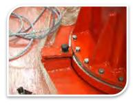
HEAVY DUTY SLEWING RING FOR SMOOTH ROTATION OF THE COLUMN
