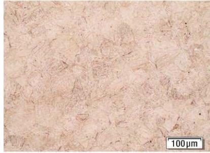
Fig. 7. Martensite formed during induction hardening (2% Nital etch, original magnification 200x). a. AISI 1080 properly IH with grain size ASTM 6. b. 4140 alloy overheated with grain size ASTM 4.
