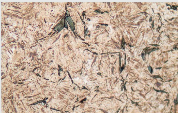
Bainite (blue-gray phase) in martensitic matrix formed due to insufficient quenching during induction hardening. The part is an AISI 1055 steel forging. Original magnification: 1000x with 2% Nital etch, taken with an Olympus GX-41 (courtesy of Induction Tooling Inc.).
