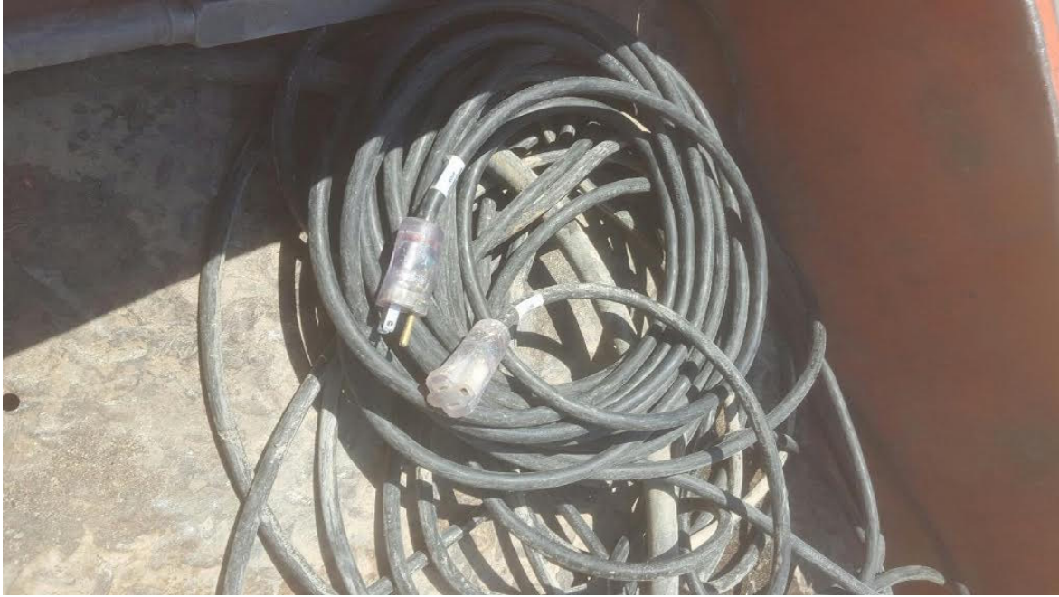
Figure 11. This Solid Ground extension cord with SJTOOW Jacket is still being used on a construction job site after 14 months of operation.
