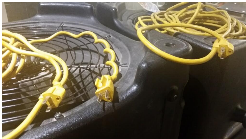
Figure 1. Three “construction grade” extension cords all with missing ground pins.
