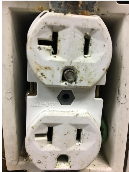
Figure 3. Conventional Ground Pin Broken off in electrical outlet.
