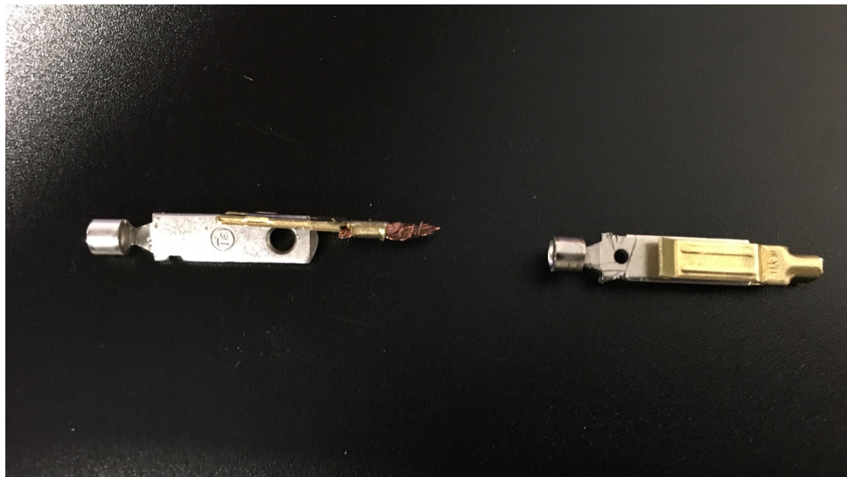
Figure 16c. Final comparison of partial clip versus full blade surface area coverage clip.
