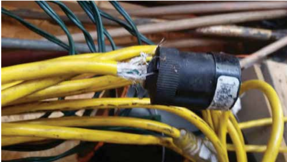
Figure 7. Conventional extension cord showing jacket separation from the plug due to an insufficient jacket retention device.
