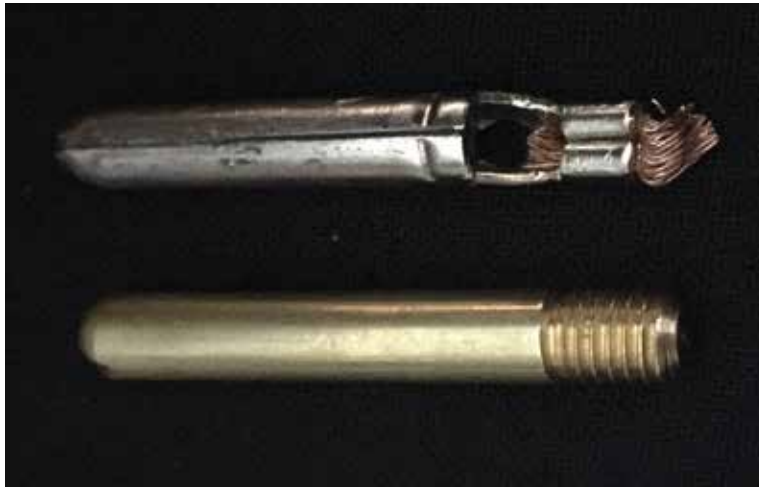
Figure 2. Anchored, solid ground pin versus conventional, hollow ground pin.
