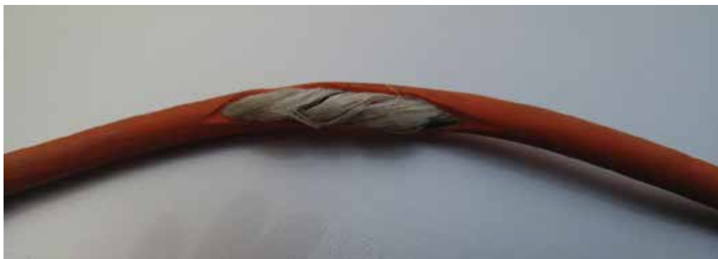
Figure 9. Conventional extension cord with a split SJTW jacket due to jacket degradation.
