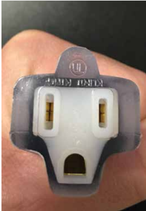
Figure 16c. Final comparison of partial clip versus full blade surface area coverage clip.
