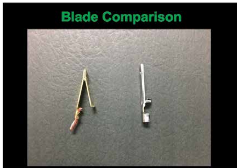
Figure 6. Thin, easily bendable, folded blades versus solid blades.
