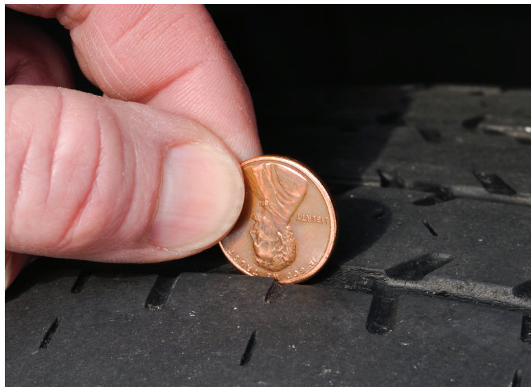
Placing an upside-down penny in any tread groove is an efficient way to check your tires' tread. If you can see Lincoln's entire head, it's time for a replacement.
